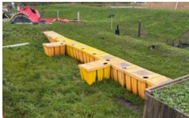
Figure 35 BoxBarrier Movable barrier mini-setup test at Flood Proof holland
