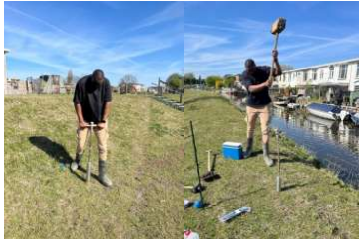
Figure 8 Shows the probes being extracted from the ground for sample collection at different locations.
