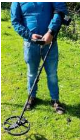
Figure 2 Nokta Simplex metal detector for cable tracing
