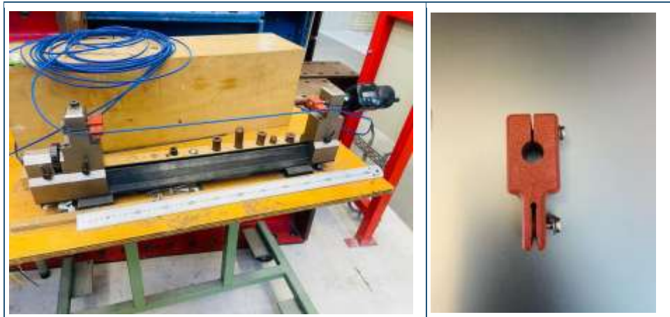
Figure 26 Strain gauge measurements for calibration of the cable
