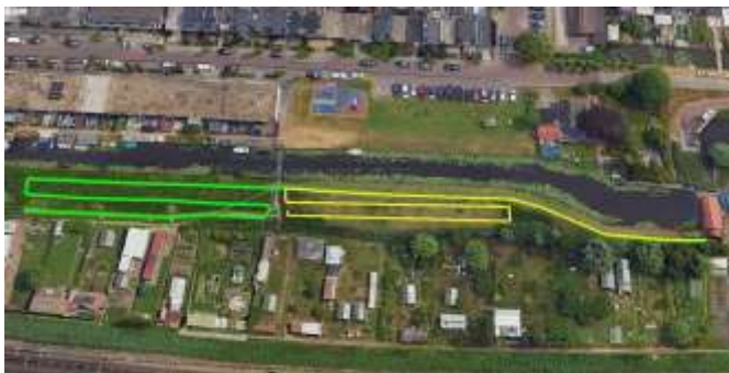
Figure 5 Exact location of the cable (in green) which was overlaid with the initial thought of the cable position.
