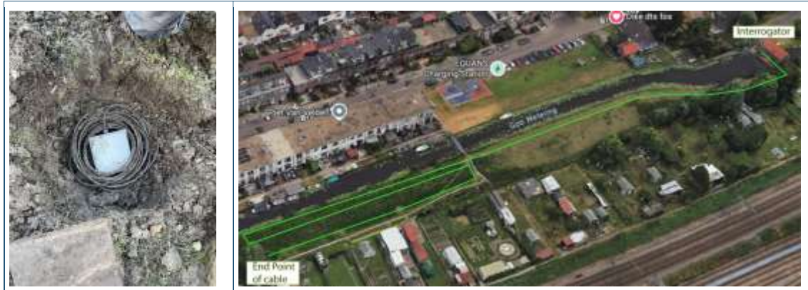
Figure 6 Left image: location of the end-point of the cable, which has a coil of cable of approximately 10 m. Right image: Interrogator location inside the pumping station.
