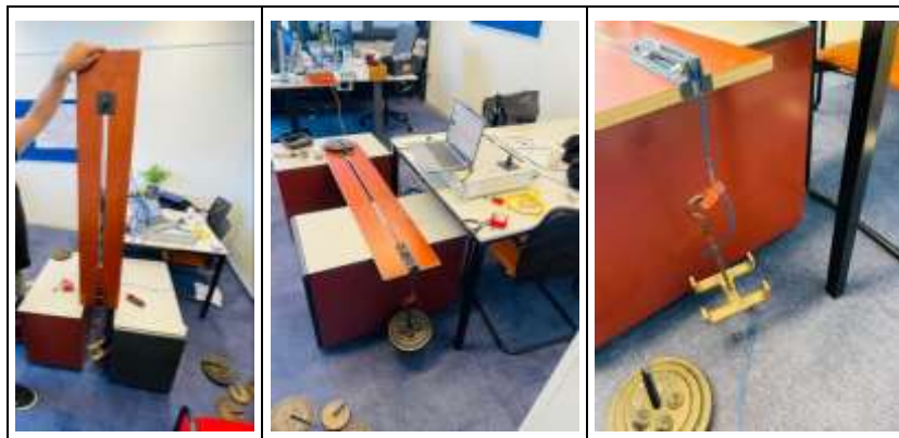
Figure 29 Vertical test, Horizontal test and loading plates of the clamp tests V1.0.
