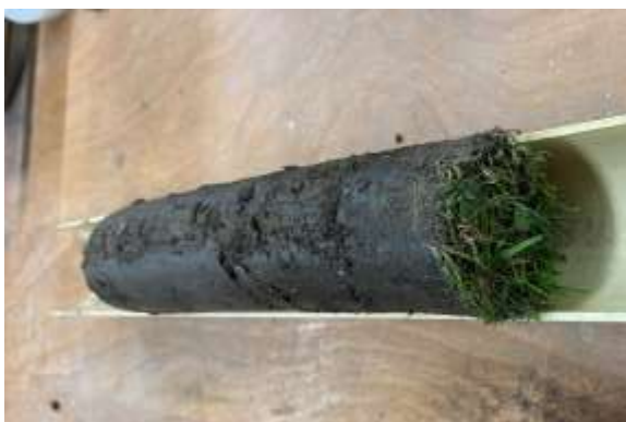
Figure 9 Shows a freshly collected sample, ready to be weighed before being dried in the oven
