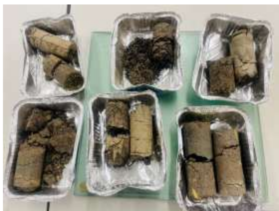
Figure 9 Shows a freshly collected sample, ready to be weighed before being dried in the oven
