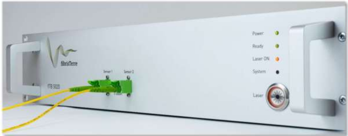
Figure 20: The interrogator (issues a laser pulse to the fiber cable for the measurement of temperature and strain) installed in the pump house for measuring temperature
