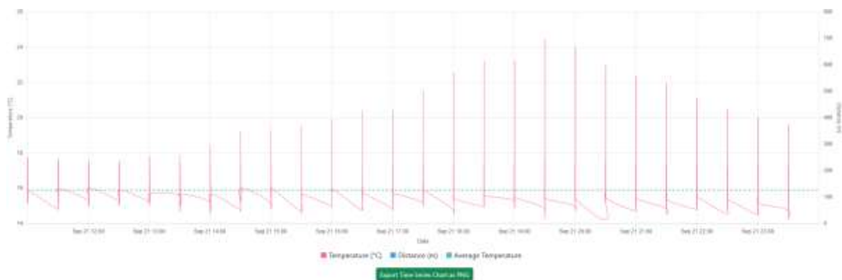
Figure 6: A time series over a period of 24 hours, showing how the temperature varied in the dike between day and night
