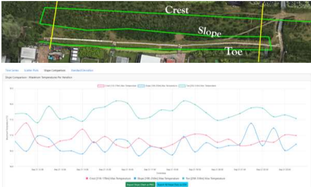
Figure 10: Isolates the temperature in the crest, slope and toe of the dike for easier understanding of the cable location in relation to the fiber distance.
