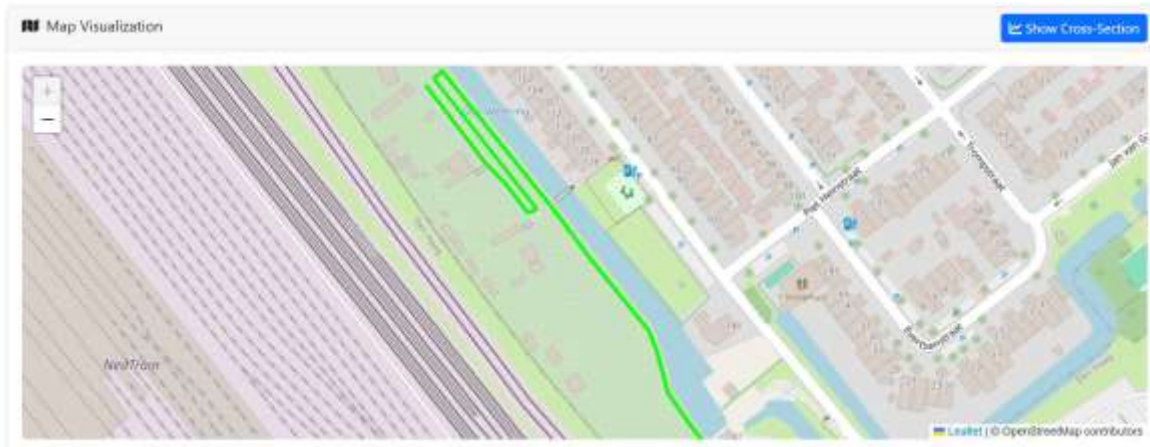
Figure 3: A map describing the precise location of the single mode fiber optic cable installed in the dike under study in Leischendam, South Holland, represented with a green continuous line.
