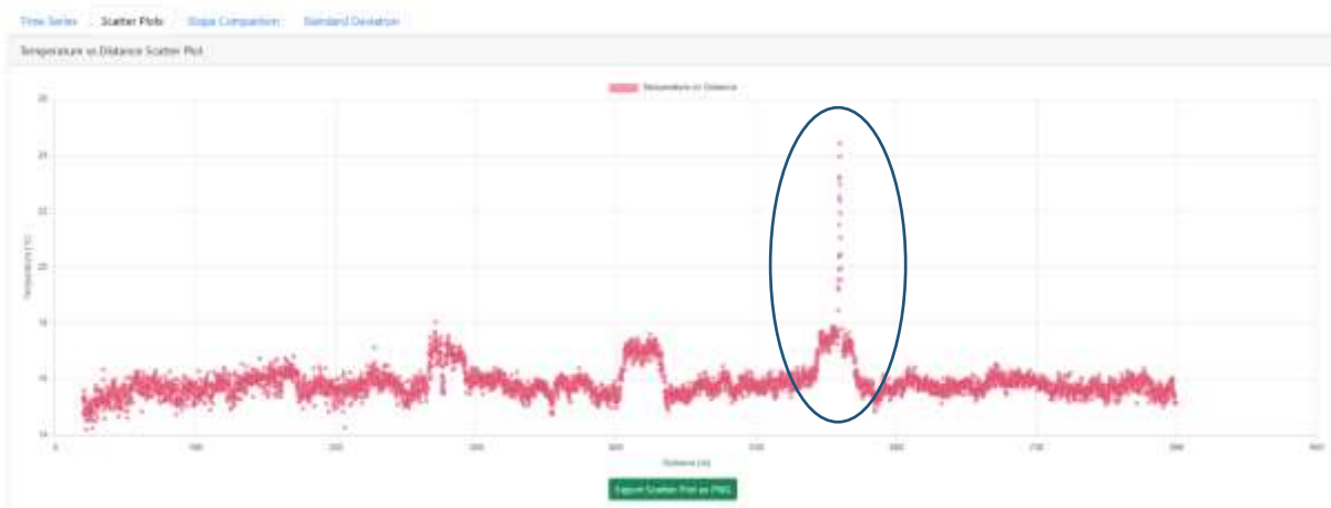
Figure 13: The outlier signal highlighted in the red circle. It was later filtered out and the signal was stabilized
