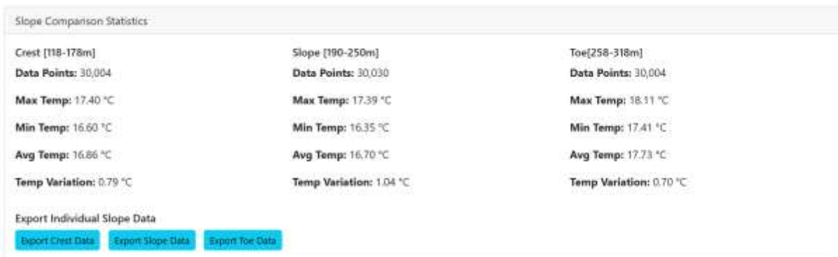
Figure 11: An analysis of the temperature variation in the crest, slope and toe of the dike to aid a quick analysis of the temperature changes in the three parts over a defined period of time.
