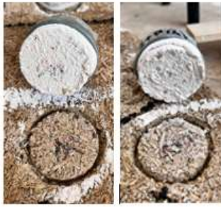
Figure 43. Failure mechanisms of HEMP+PAINT (pictures courtesy of UNIVPM).
