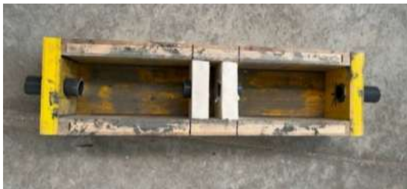
Figure 23 Mould with PVC tubes and polystyrene pieces (picture courtesy of UNIVPM).
