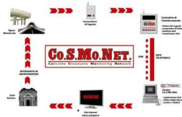
Figure 28 Co.S.Mo.Net monitoring system (picture courtesy of UNIVPM).
