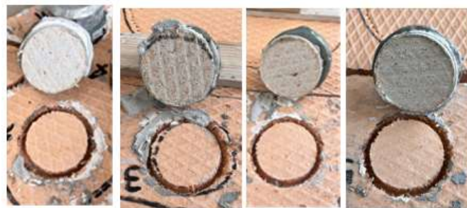
Figure 42. Failure mechanisms of XPS+UNIVPM (pictures courtesy of UNIVPM).
