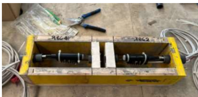
Figure 25 Mould with electrode array, TiMMO electrode, and steel rebars (picture courtesy of UNIVPM).
