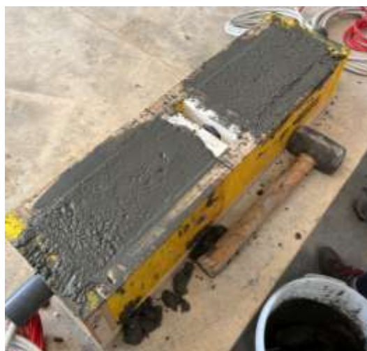
Figure 30 Specimen just after the pouring phase (pictures courtesy of UNIVPM).
