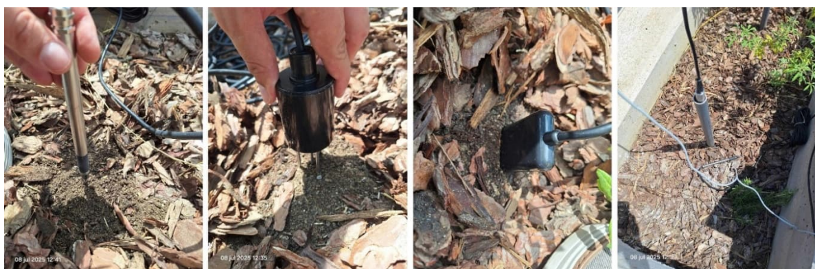
Figure 26. Sensors installed to indirectly evaluate the biofilter stormwater management. From left to right: EC/salinity sensor, soil moisture sensor, soil temperature and humidity sensor, and piezometer. Source: MULTICLIMAT
