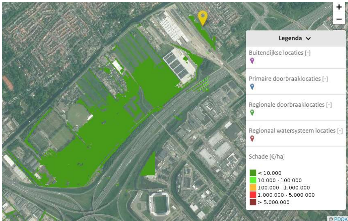
Figure 20. Damage Estimation Based on Simulated Flood Depths, Showing Expected Monetary Damage Below €10,000 per Hectare and Total Estimated Damage of €19 Million per Year.
