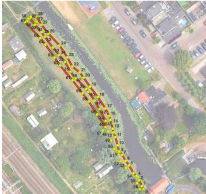
Figure 32. Aerial view of Tedingerbroek dike and the mapped location of the embedded fiber optic cable. Source: (Aguilar-López, Nöter, and Inghosso 2024)
