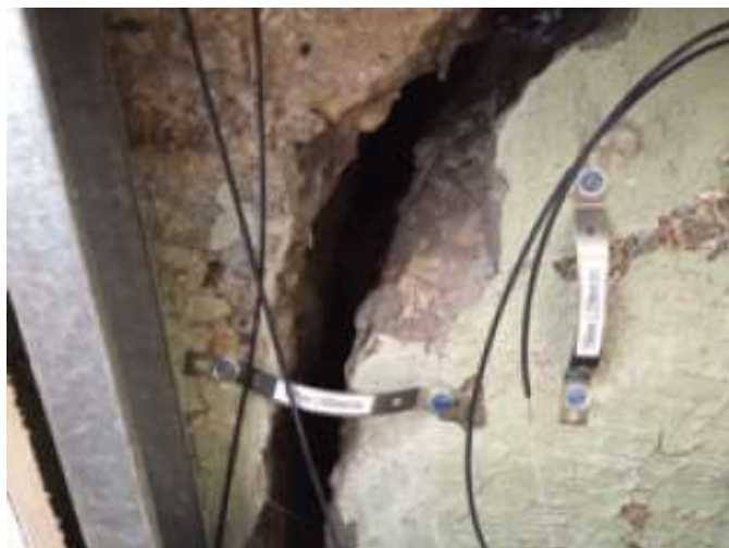
Figure 26: Example of FBG crack sensors applied to cracks.
