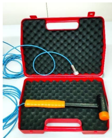
Figure 80: sonic velocity instrumentation (instrumented hammer for measuring sonic velocity).
