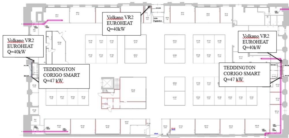
Figure 5 Location of air curtains and hot air blowers in the dairy pavilion building
